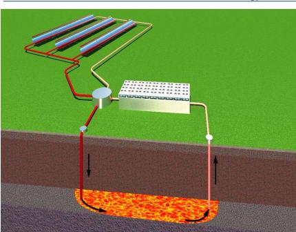
RenewGeo technology is about creating a synthetic geothermal storage resource by heating a natural brine with solar energy and adding enough heat when the sun shines to generate power 24 hours a day.
